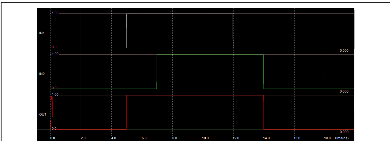
Figure 3.8. OR Gate simulation in Microwind35
