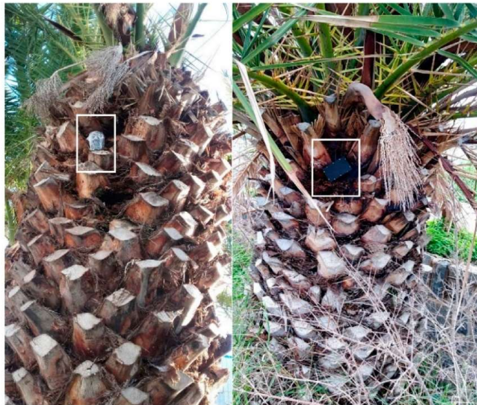
Figure 9-26. Operating in transmission mode. The device attached to a palm tree listening for R. ferrugineus . The white rectangle is located around the device. The recordings bearing a time-stamp are uploaded to system server where the user can examine them and download them.
