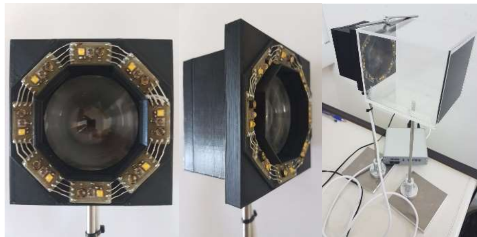
Figure 2-5. Prototype of the multispectral sensor.
