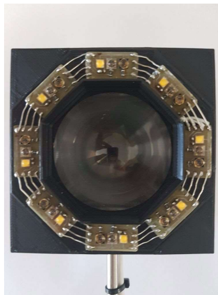
Figure 3-1. The multispectral sensor: The disk in the middle is the Fresnel lens. The three LED's in each plate emit, in turn, visible light 450-700nm, and infrared at 810 nm and 940 nm. All eight LEDs of each spectral band are lit simultaneously and each band switches in turn every 20.8 microseconds. All LED plates have 68.5o with respect to the Fresnel plane;
