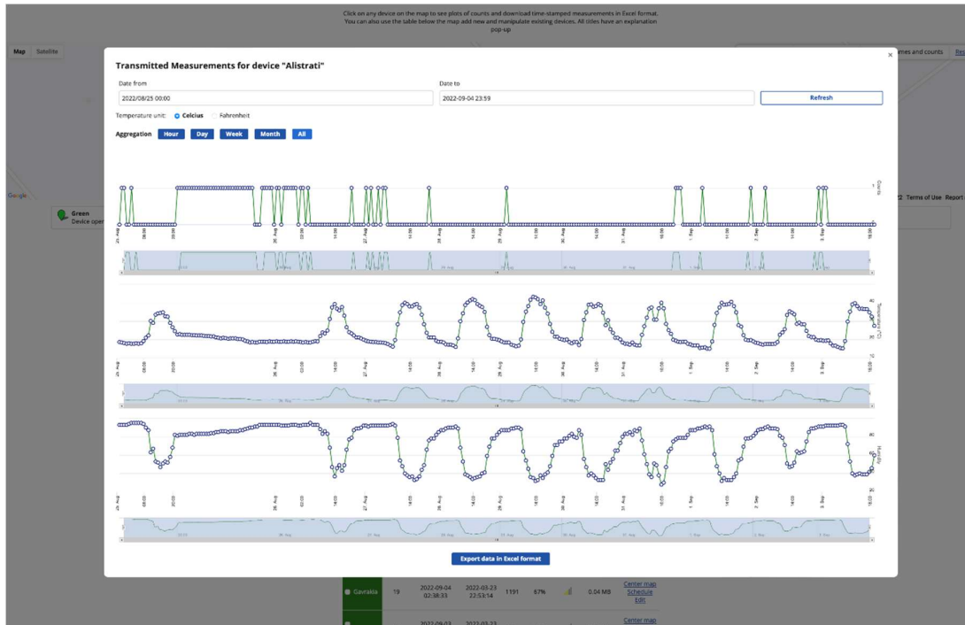
Figure 9-48. A Pop-up window will appear when someone clicks on device’s icon. On the map in system server. View report leads to a window where temperature and a number of clips per day are plotted. The user sees a time-series of counts, collective counts and associated temperature recordings. All information can be downloaded by clicking the ‘Export data in Excel format’ tab.
