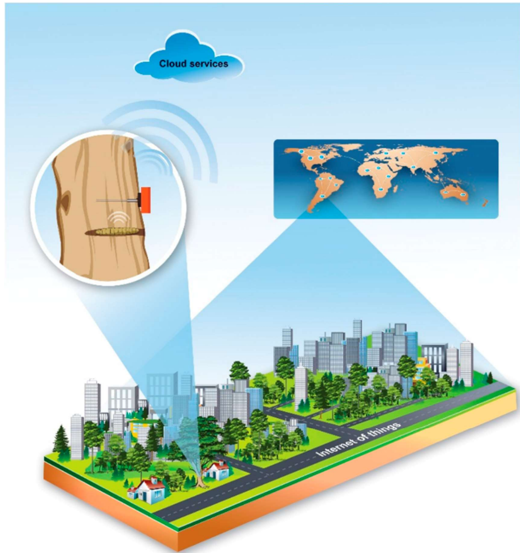
Figure 5-1. The concept of acoustic surveillance of trees in forests and urban environments.
