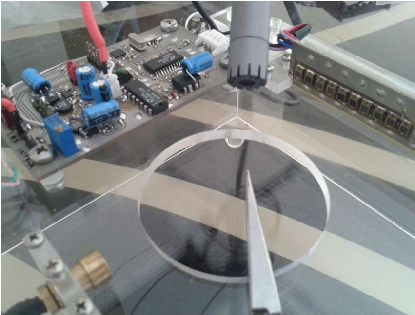
Figure 2-20. In-flight recording from the optoacoustic device. a) The laser emitter and the beam splitter attached to the emitter, b) small aperture gun microphone, c) array of photodiodes. The cross-lock tweezer in the middle holds insects by their legs
