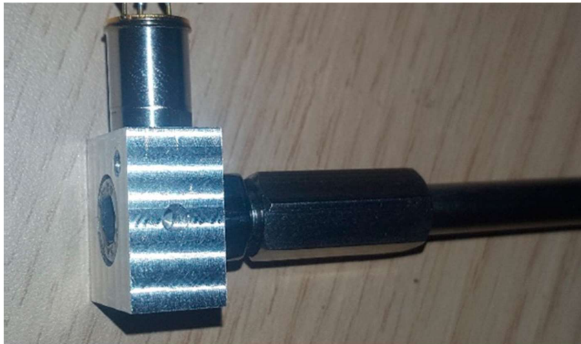
Figure 5-3. Metal waveguide fastened to the input of the accelerometer. The tree trunk is first drilled using a bit matching the size of the probe and the waveguide is subsequently inserted and fastened in the hole.
