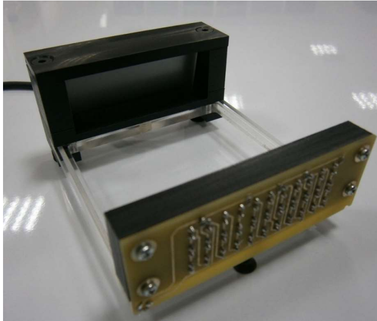
Figure 2-30. The sensor The light-guide aperture inside a dark box providing shade and sitting on 1D array of diodes
