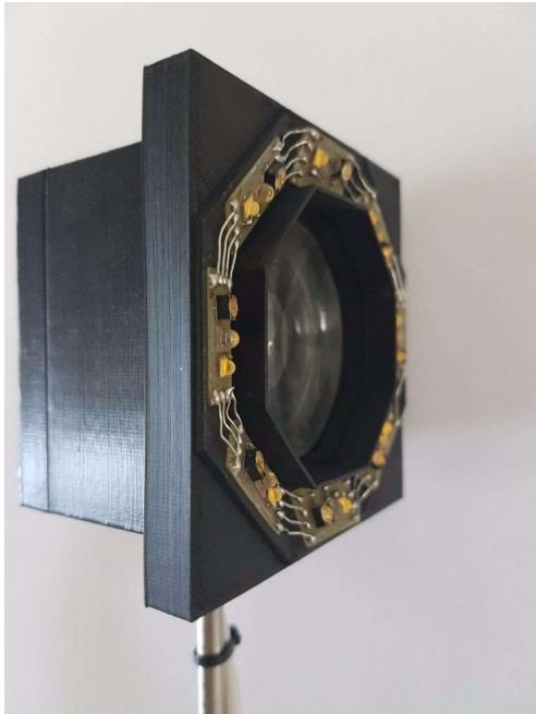
Figure 3-2. The photodiode is placed at the focal point of the Fresnel lens.
