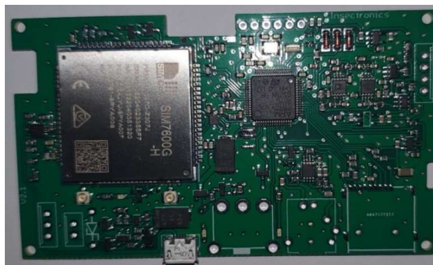
Figure 9-39. Assembled PCB (SMT components only)
