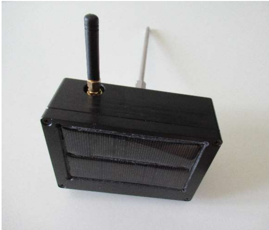
Figure 9-23. For outdoor operation, the device has a solar panel on its back.
