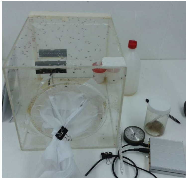
Figure 2-31. 2D array of photodiodes sensor and system in their final position in an insectary cage.
