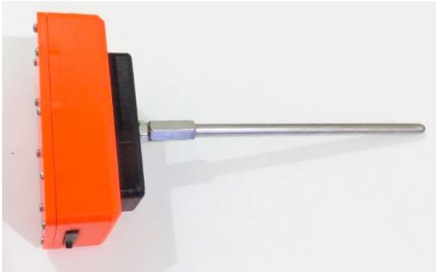
Figure 5-2. The vibrations recorder A rugged container for outdoor deployment contains the electronics including GPS and 4G-LTE communication.
