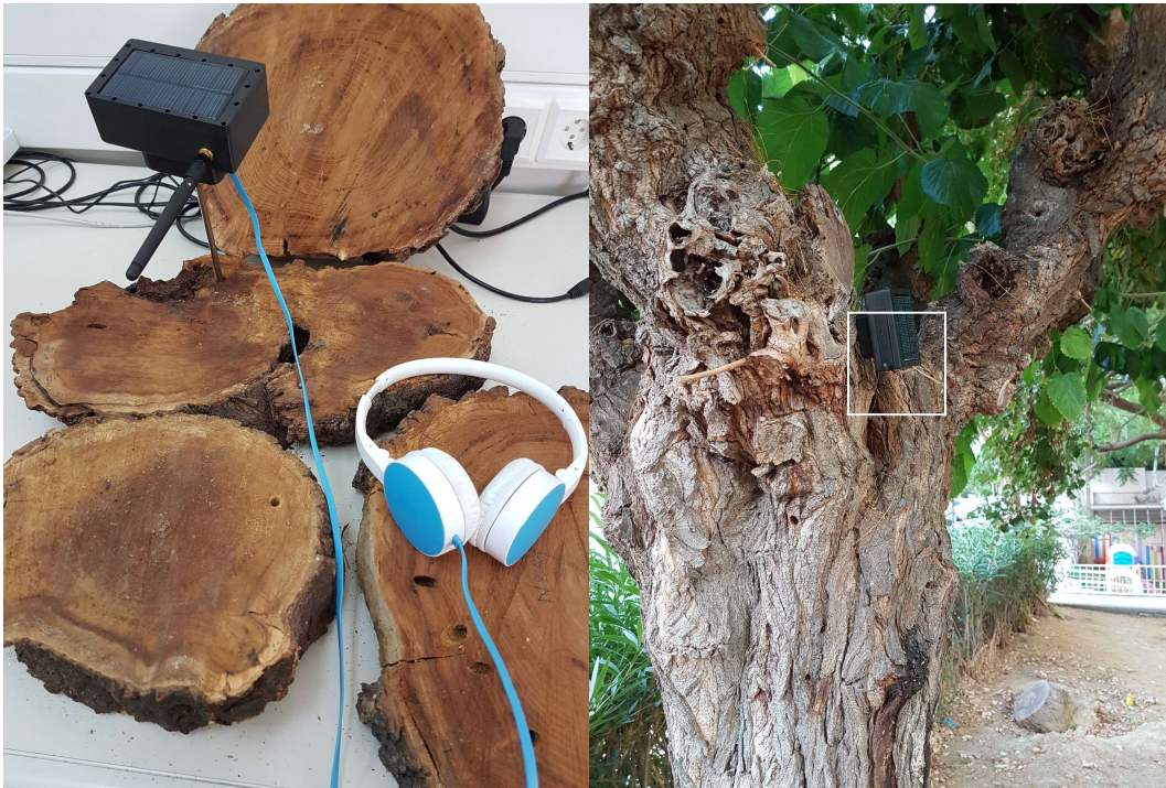
Figure 9-25. Operating in continuous output mode. The user examines the internal activity in the trunk through the headphones, (Left) Manual inspection of slices of a trunk. (Right) Remote examination of tree in the field.
