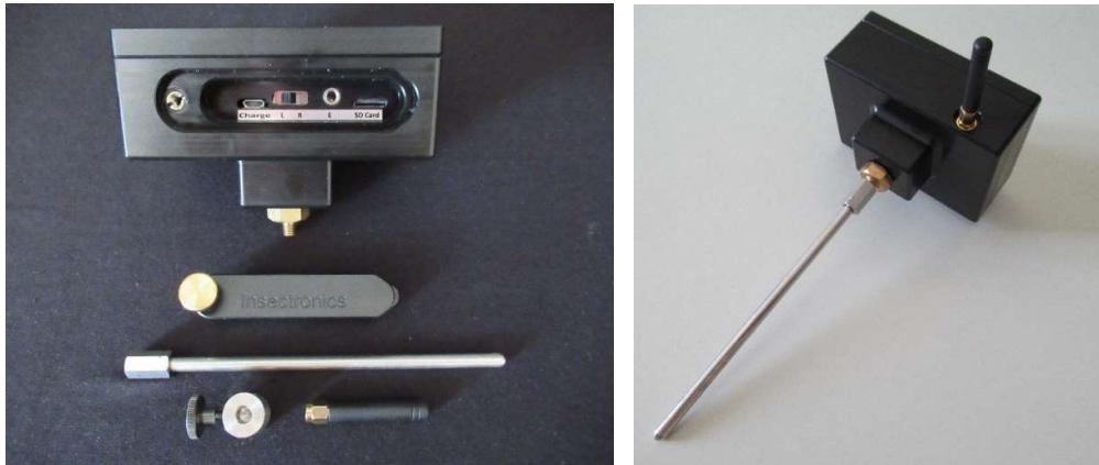
Figure 9-20. Complete tree vibes system (Left) The main black box (10.8cm X 6.8cm X 6.8cm) contains the electronics and the SD card. A communication antenna, a waveguide and an adapter can be seen. The device has an embedded solar panel connected to its battery. (Right) The assembled device.
