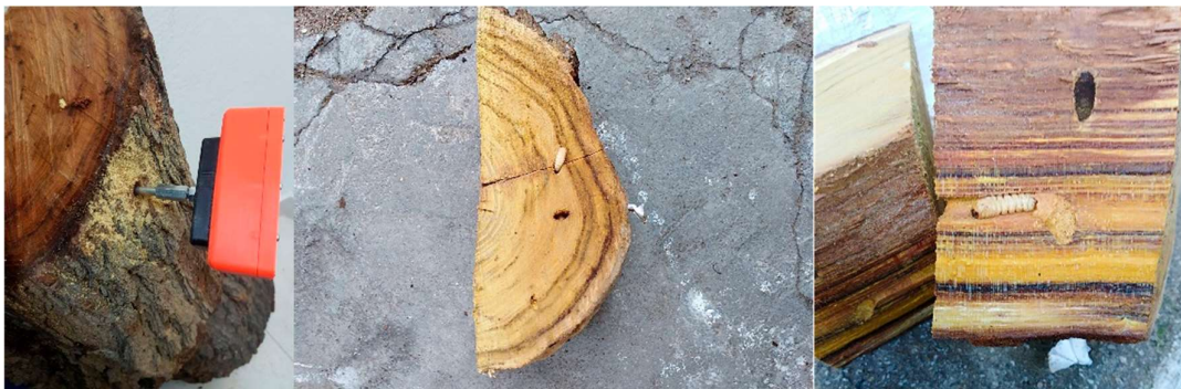
Figure 5-13. A X. chinensis positive case in a mulberry trunk. (Left) The sensor mounted horizontally in a suspicious trunk in the laboratory, (middle and right) two alive larvae have been found after cutting the suspicious trunk in slices. The larvae tunnels can be seen in the right picture.
