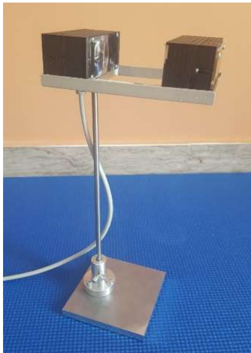
Figure 2-3. A prototype of the extinction light sensor.
