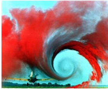
Figure 1.19. Vortex created by the passage of an aircraft wing, revealed by colored smoke
