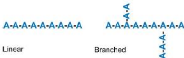
Figure 1.1 Schematic representation of a homopolymer.
