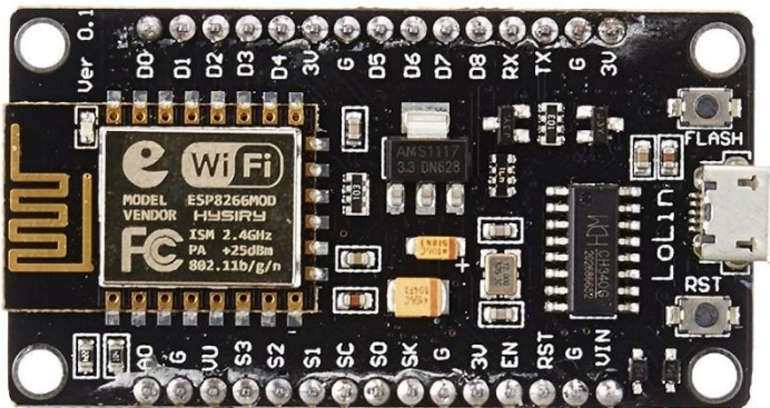
(Σχήμα 4.3.4 NodeMCU ESP8266, έχει 8Mbytes flash memory, 128kBytes RAM, 160 MHz clock speed, 16 I/O pins, 1 analog input, 32-bit RISC architecture)
