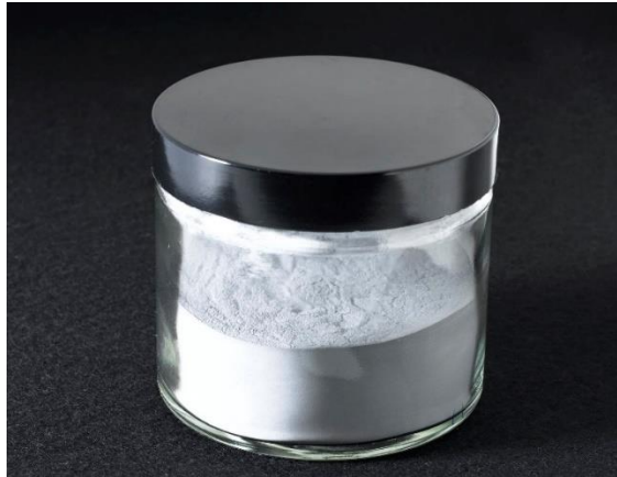
Σκόνη Αλουμινίδης-Νικελίου. Πηγή: "Sample of Nickel aluminide powder, used as a catalyst (sample of nickel aluminide)" by CERAM is licensed under CC BY-NC-SA 4.0
