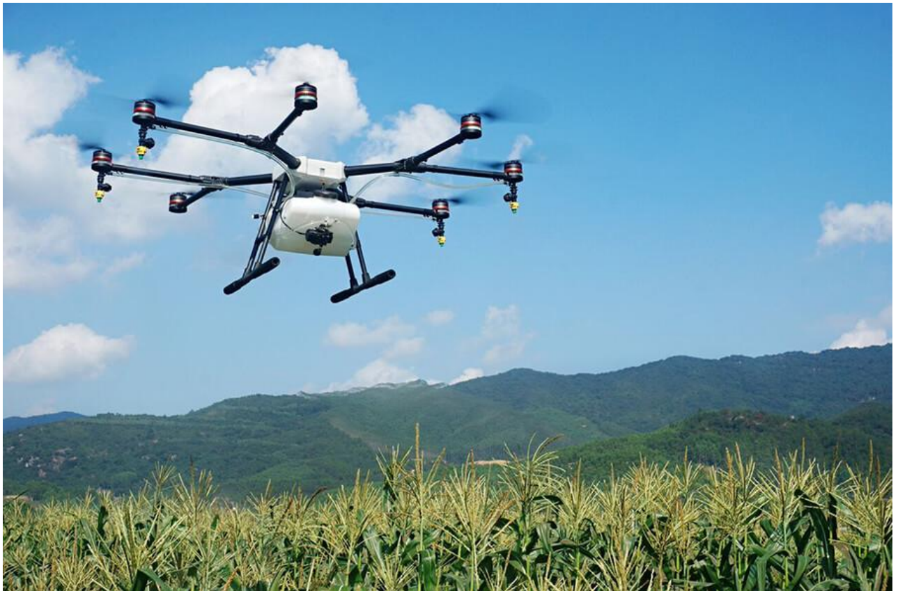
[47] Rotary wing UAV with a tank that can spray liquids.
