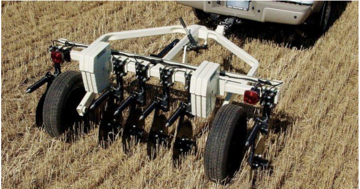
[49] A sensor that measures the electrical conductivity of the soil while the tractor is moving.
