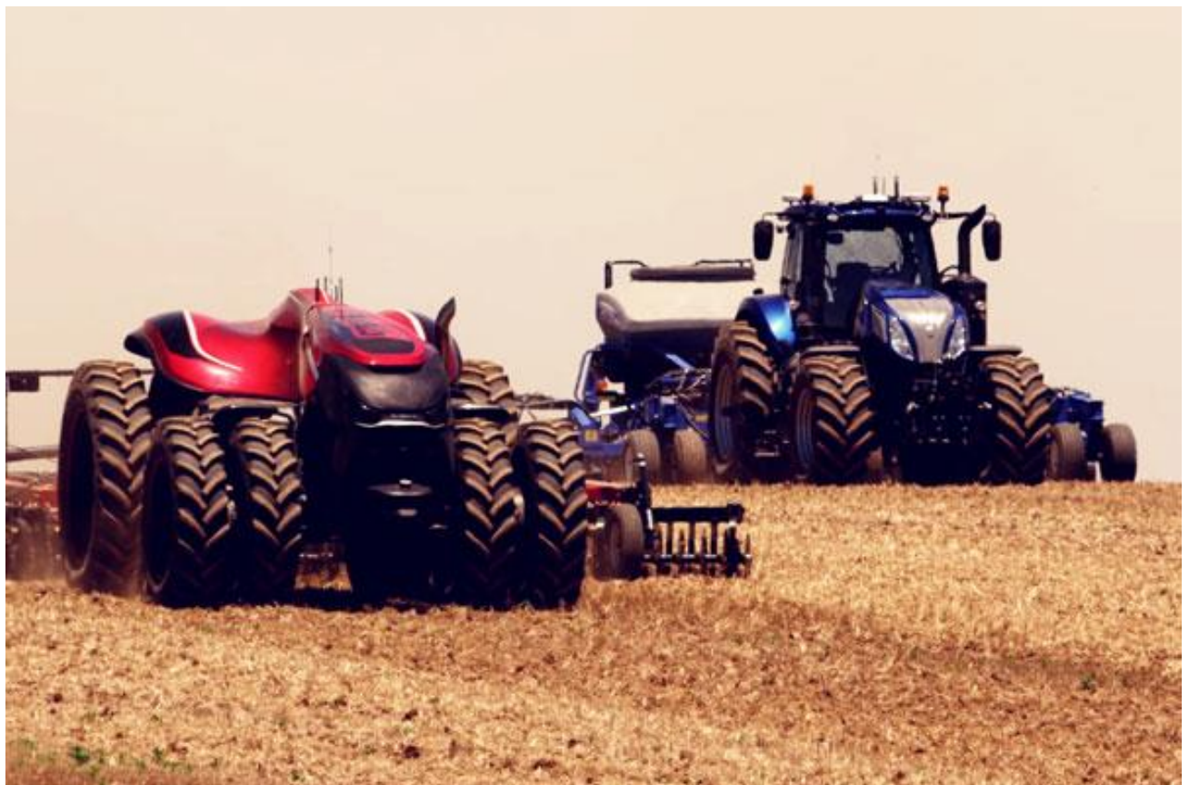
[48] An autonomous and a semi-autonomous (there is no driver to the blue tractor) collaborating.
