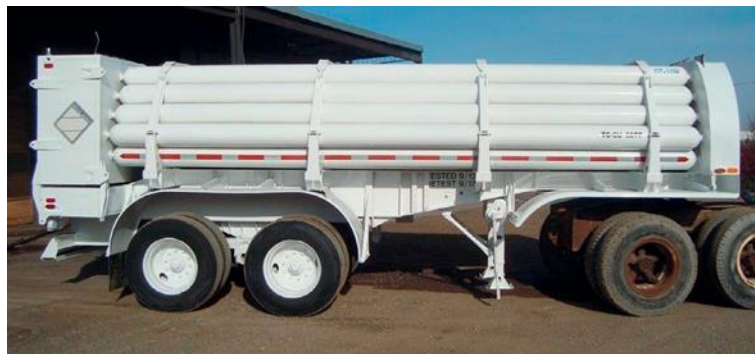
Figure 29. Hydrogen tube trailer.
