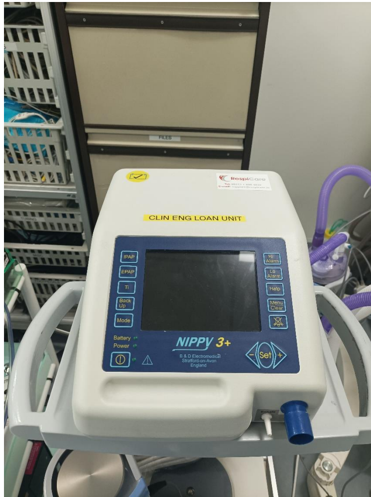
Figure 5. A NiPPV ventilator from RespiCare
