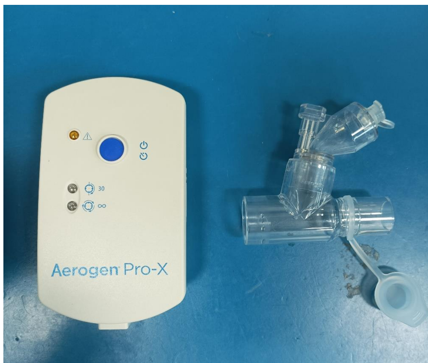
Figure 7. Mesh nebulizer from Aerogen Ltd.
