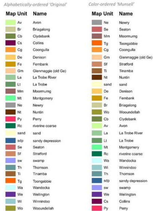
Figure 24: Alphabetical-Ordered (Left) and Color-Ordered Legend (Right) Legend Designs of Soil-Landscape Maps Used in Experimental Research Study (Source: Çöltekin, et al., 2017)
