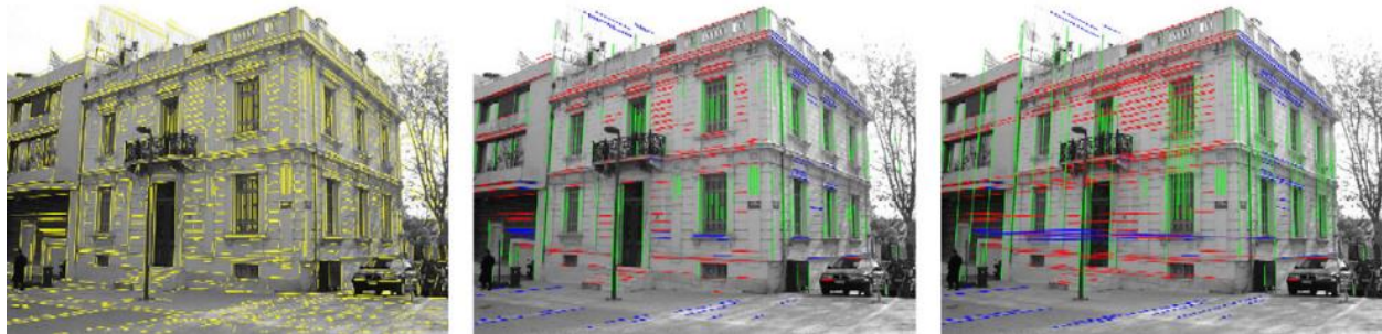
Figure 14: Left: Extracted edges, Middle: Vanishing lines, Right: Vanishing lines after lens distortion correction, by (Grammatikopoulos et al., 2007)
