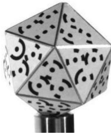
Figure 10: Example of 3D calibration object by (Forbes et al., 2002)
