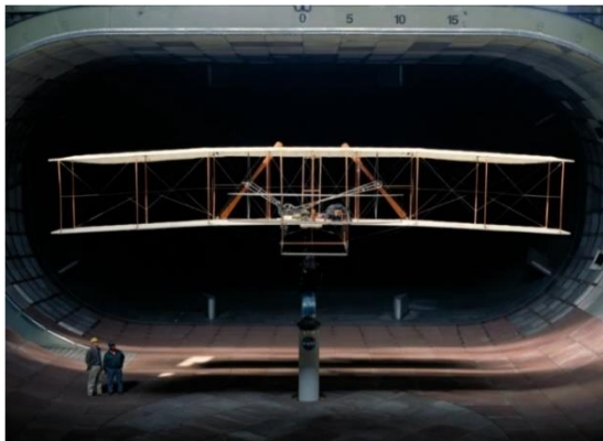
Figure 1.2 Wind tunnel testing of Wright brothers' airplane (NASA, 1999)
