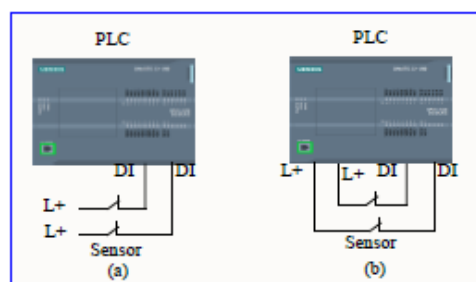
Fig. 4: Sensor wiring with double channels (1oo2)
