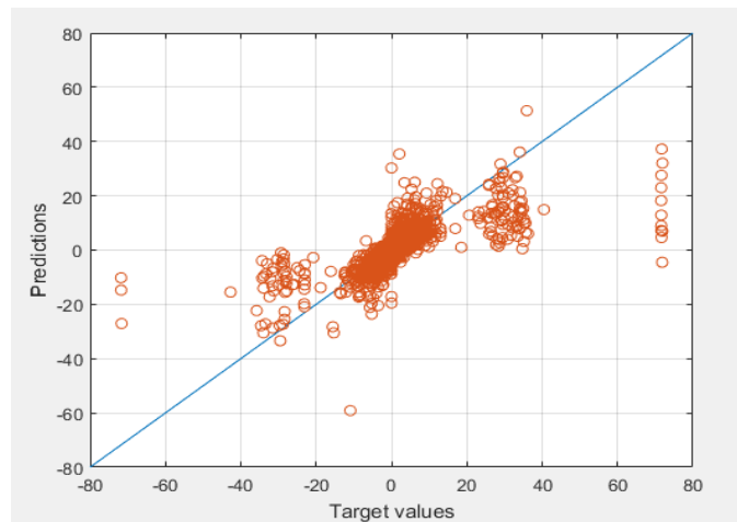
Figure 11: Target values vs Predictions of RBFs using the proposed features with mating evaluation filtering
